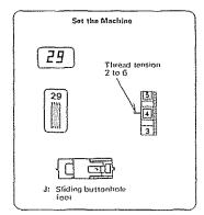
The Kenmore 100 Stitch automatically dams rips and holes. Large and small holes can be mended quickly and easily with this unique stitch.
